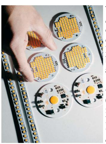
We offer line voltage and low voltage LED modules—efficient solutions to effectively provide the same light quality as halogen bulbs—which we design and manufacture.
