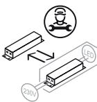
EN The LED driver contained in this fixture must only be replaced by the manufacturer, its support service or similarly qualified personnel.
