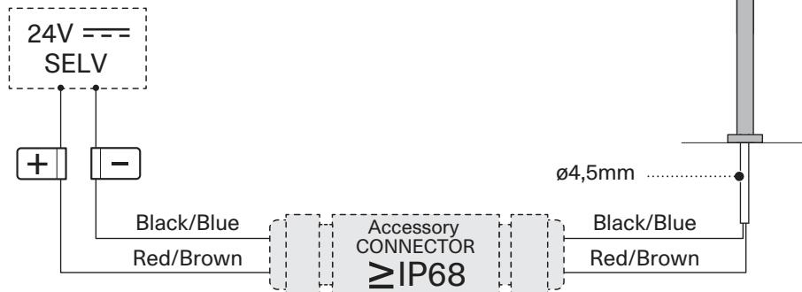
The connection system must comply with the installation conditions and, in any case, must have a protection rating that is at least equivalent to that of the appliance. It must also be compatible with the type of cable used in the appliance, in accordance with current regulations.
