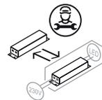
EN The LED driver contained in this fixture must only be replaced by the manufacturer, its support service or similarly qualified personnel.
